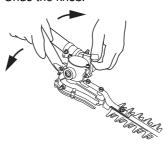
Press the cutting head against the ground or some other solid object until the desired angle has been obtained.
